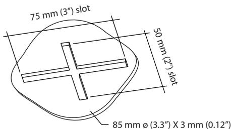
Figure 2 Insulation Support/Retainer
