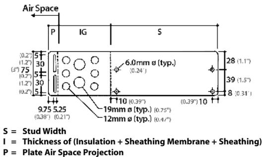
Figure 1 Slotted Stud Plate (Type II)
