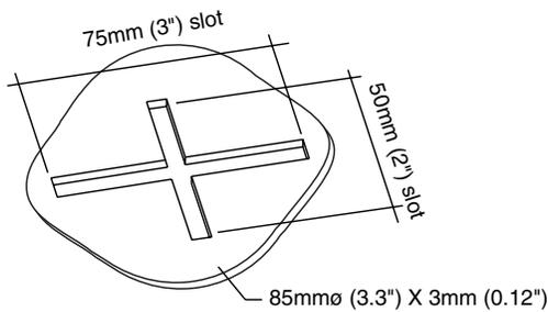
Figure 3 Insulation Support/Retainer
