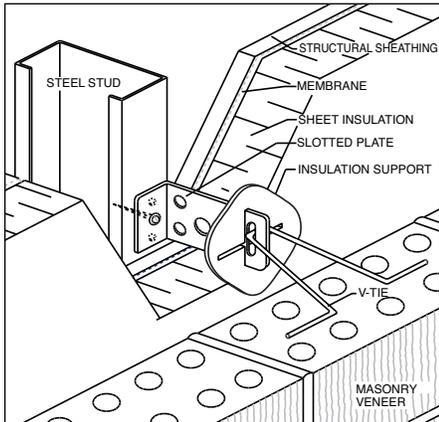
Figure 4 Slotted Heavy Duty Rap-Tie Attached Directly to a Steel Stud
