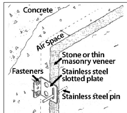
Figure 6 Slotted Heavy Duty Rap-Tie System Application for Dimension Cut Stone Veneer
