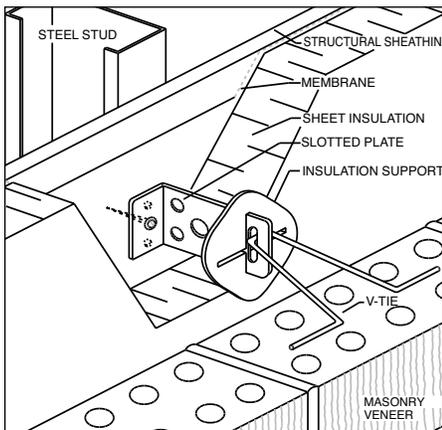
Figure 5 Slotted Heavy Duty Rap-Tie Surface Mounted on Protected Structural Sheathing
