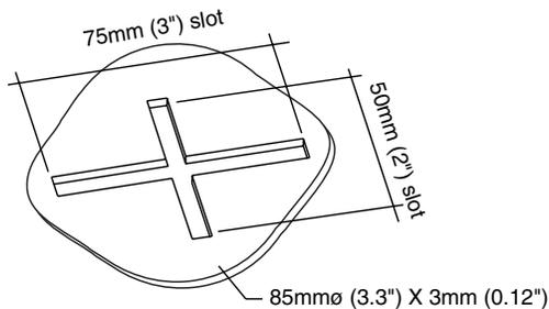
Figure 3 Insulation Support/Retainer
