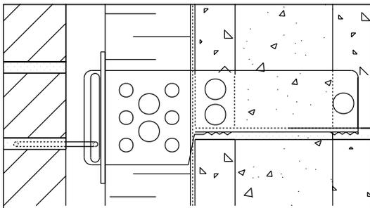
Figure 5 Slotted Block Tie (Type I) Installation
