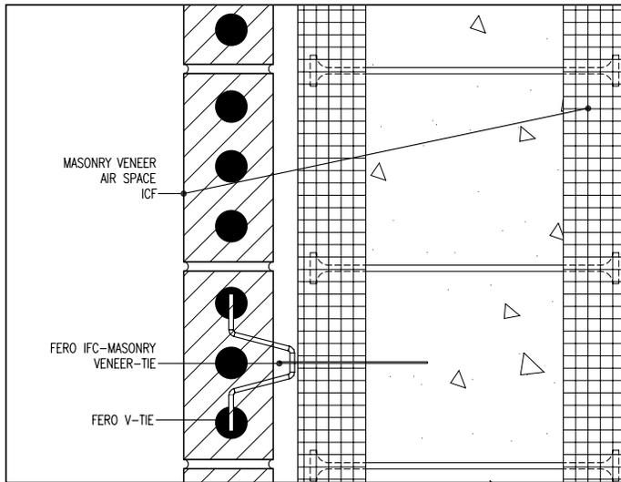
Figure 3 - Plan showing the V-Tie and Veneer
