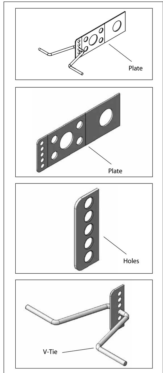
Figure 4 - Components and Installation Sequence
