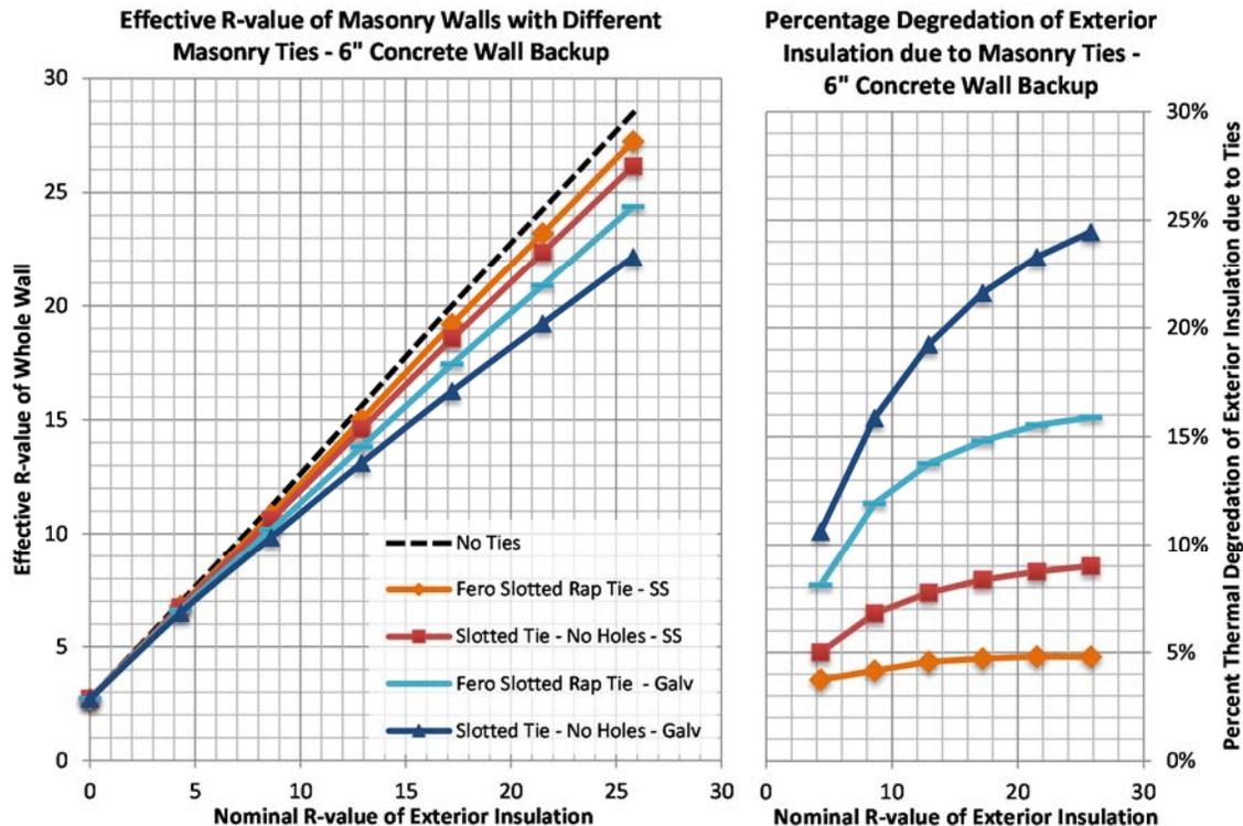
**Figure 2: Effective R-value and Corresponding Percent Thermal Degradation of Masonry Walls with Different Masonry Ties - 6" Concrete Wall Backup**
