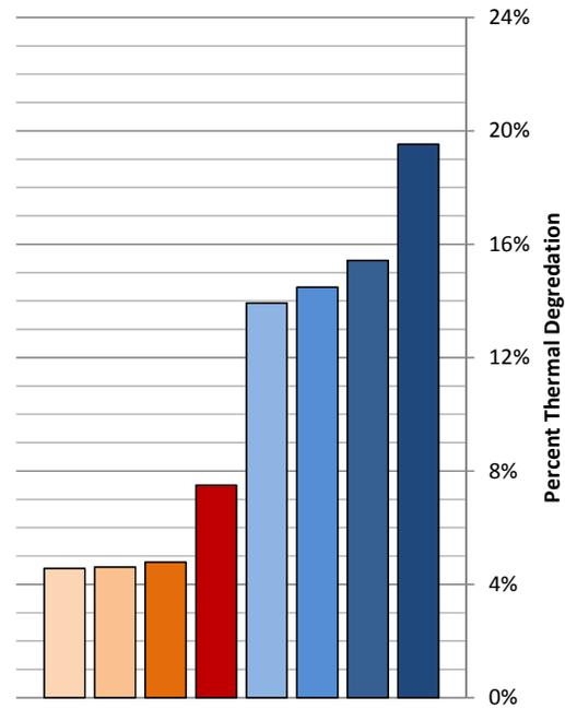
**Figure 6: Effective R-value and Corresponding Percent Thermal Degradation of Masonry Walls with Different Ferro Rap Ties and Installation Modifications – 3 5/8" Steel Stud Wall Backup**
