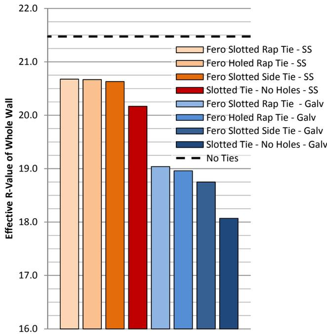
**Percent Degredation of Exterior Insulation due to Masonry Ties - Uninsulated 3 5/8" Steel Stud Backup with 4" Exterior Insulation**
