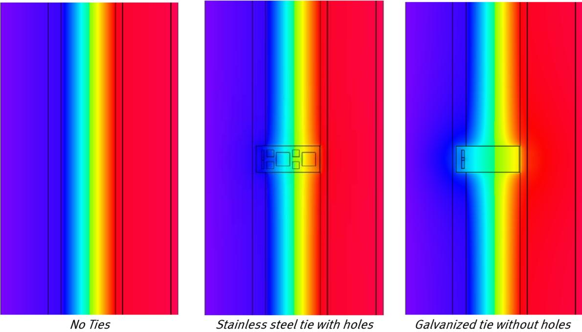
**Figure 5: Relative temperature gradient across a masonry veneer wall at a section without ties, a stainless steel tie, and a galvanized tie without holes.**
