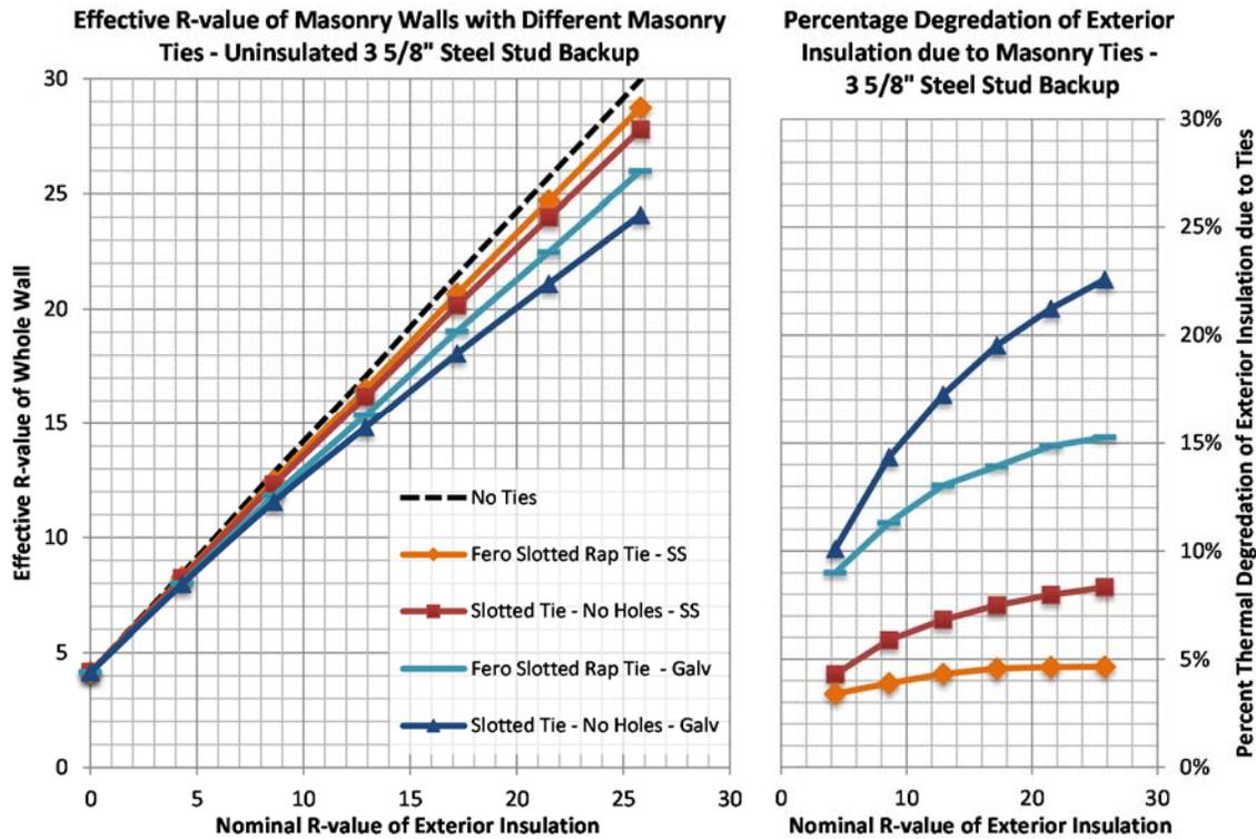
Figure 3: Effective R-value of Masonry Walls with Different Masonry Ties - Uninsulated 3 5/8" Steel Stud Wall Backup
