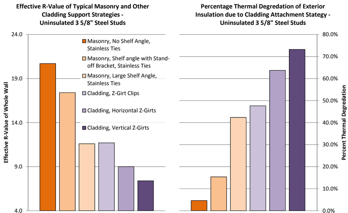
**Figure 9: Effective R-value and Corresponding Percent Thermal Degradation of Typical Masonry and Other Cladding Support Strategies – 4" exterior insulation over uninsulated 3 5/8" steel studs**
