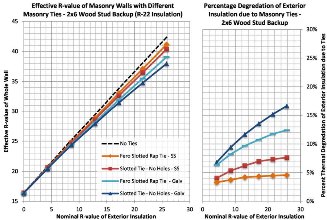
Figure 4: Effective R-value and Corresponding Percent Thermal Degradation of Masonry Walls with Different Masonry Ties - 2 x 6 Wood Stud Wall Backup (R-22 Batt Insulation)
