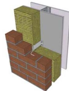
*Standard face mount 2 inch 16 gauge masonry tie (no punched holes)*
